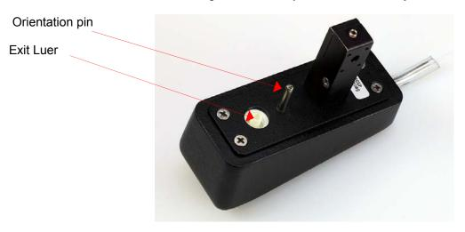
Figure 1.5.5.1-3 Bottom of flowcell assembly
