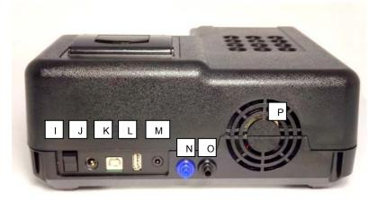
Figure 1.5.4-5 Ports and Connections
