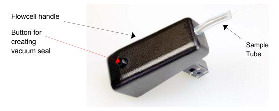
Figure 1.5.5.1-2 Top of flowcell assembly
