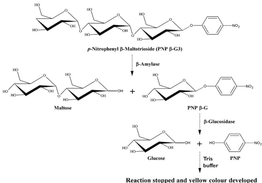
**Scheme 1. Theoretical basis of the Betamyl-3<sup>®</sup>  $\beta$ -amylase assay procedure.** When PNP $\beta$ -G3 is cleaved to maltose and PNP $\beta$ -G, the latter is rapidly cleaved to *p*-nitrophenol and glucose by the excess quantities of  $\beta$ -glucosidase which is an integral part of the reagent mixture.
