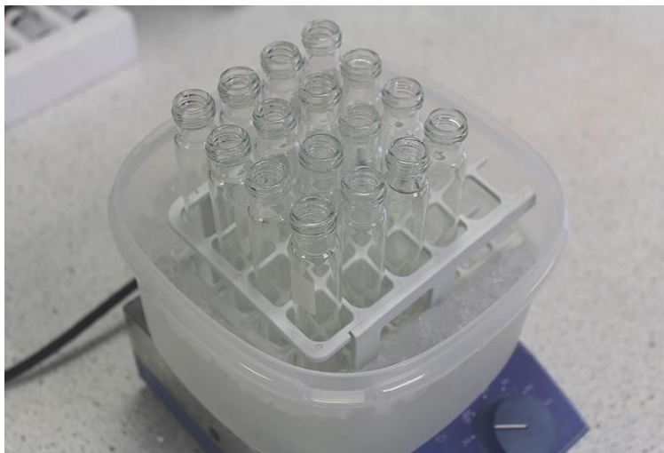
Figure 2. Arrangement of test tube racks with tubes in a rack in an ice-water bath over a magnetic stirrer for dissolution of resistant starch in 1.7 M NaOH; method (b).
