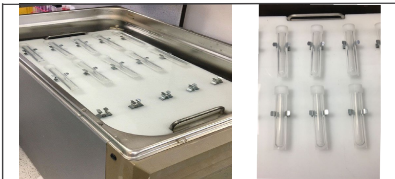
Figure 1. Attachment of 13 mL polypropylene tubes to a custom-made polypropylene tube-holder in a Grant OLS 200 water bath.
