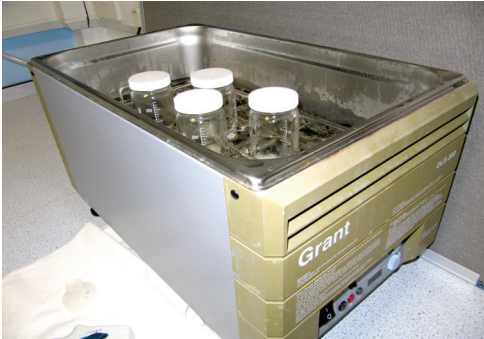
Figure 3. Picture showing mixing of samples (in rotary motion) in a Grant® OLS 200 shaking incubation bath at 37°C.
