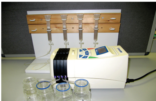
Figure 7. Deionisation of samples with mixed bed resin [ \sim 4 g Amberlite ® FPA53 ( \text{OH}^- ) and \sim 4 g Ambersep ® 200 ( \text{H}^+ )] in Bio-Rad, Econo-Pac ® Disposable Chromatography Columns connected to a Gilson Minipuls ® Evolution pump.
