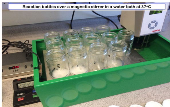
Figure 3. Incubation Method 2. Samples (~ 1.0 g) in Fisherbrand bottles on a 2mag Mixdrive 15® submersible magnetic stirrer in a water bath. This arrangement allows stirring of 15 samples at a controlled speed (170 rpm) and 37°C.
