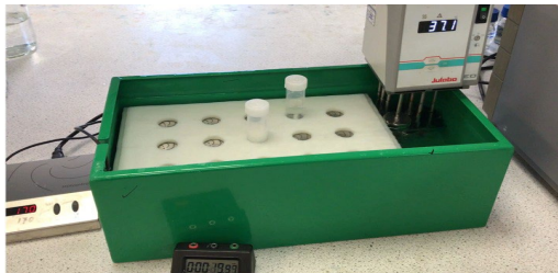
Figure 2. Incubation Method 1. Samples (~ 0.5 g) in 40 mL, 30 x 84 mm polypropylene tubes in a 2mag Mixdrive 15® submersible magnetic stirrer in a water bath. This arrangement allows stirring of 15 samples at a controlled speed (170 rpm) and 37°C.
