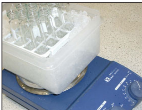
Figure 1. Arrangement of ice-water bath over a magnetic stirrer for dispersion/dissolution of sample material in 60% sulphuric acid.
