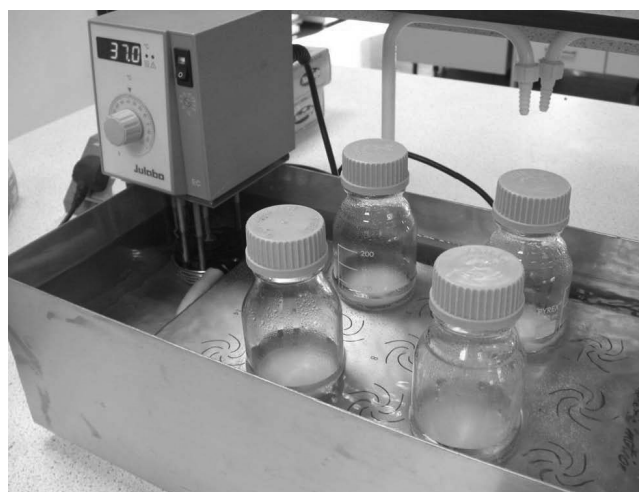
Figure 2011.25A. Typical arrangement for sample mixing using a 2 mag Mixdrive 15 submersible magnetic stirrer in a custom made water bath.
