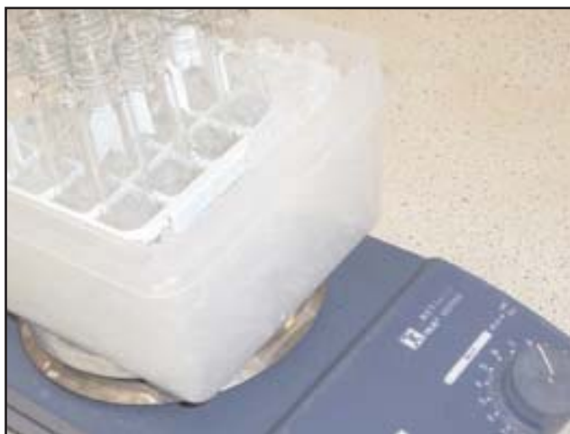
Figure 1. Arrangement of ice-water bath over a magnetic stirrer for treatment of samples with 2 M KOH and dissolution of starch and phytoglycogen.
