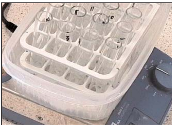
Figure 1. Arrangement of ice-water bath over a magnetic stirrer for treatment of samples with 2 M KOH and dissolution of RS.
